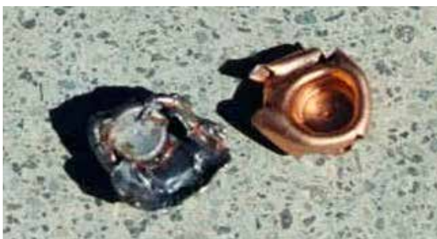
Jacket/core separation – Sierra GameKing
