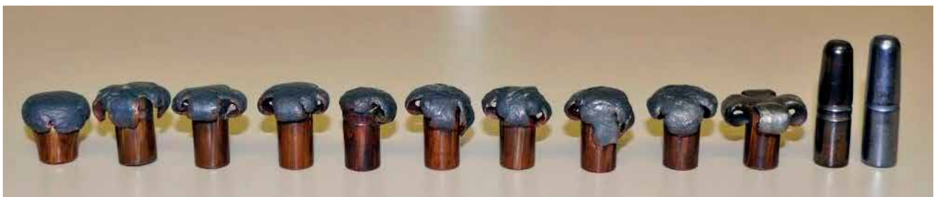
Left: .458 Rhino Bullet construction – a big-game bullet Right: A 500 gr Rhino Bullet retrieved from a lion – sterling performance, considering that it travelled through the animal lengthwise.
