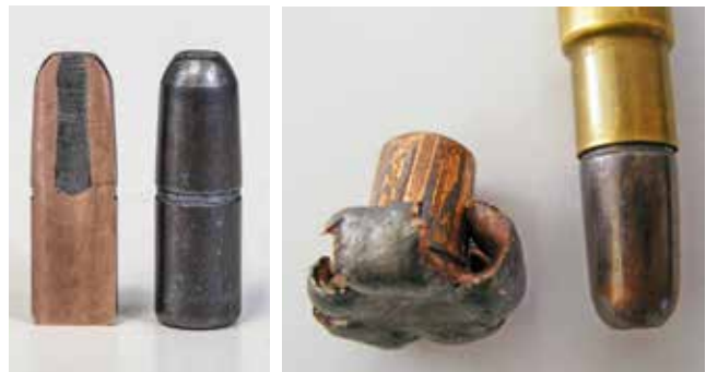
Left: .458 Rhino Bullet construction – a big-game bullet Right: A 500 gr Rhino Bullet retrieved from a lion – sterling performance, considering that it travelled through the animal lengthwise.
